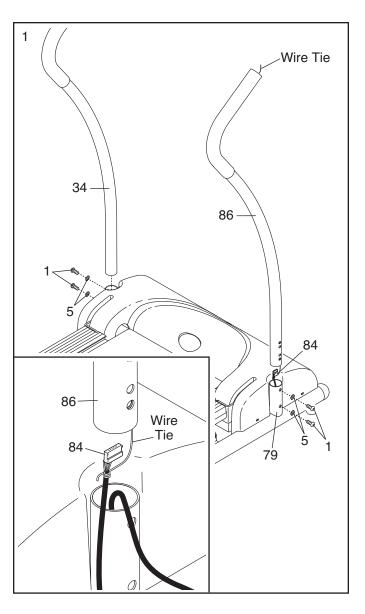
Orient the Handrail Crossbar (83) as shown. See the inset drawing in step 1. Tie the wire tie in the Handrail Crossbar securely around the end of the Wire Harness (84). Then, pull the other end of the wire tie until the Wire Harness is routed completely through the Handrail Crossbar.
